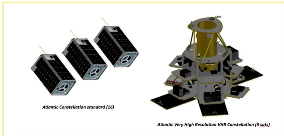
*Fig. 4 - Concept small satellites: 20kg platform - 16 satellites & platform 80kg - 3 satellites*
