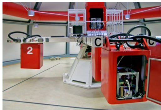
The Large Diameter Centrifuge at the European Space Research and Technology Centre Credit: ESA
